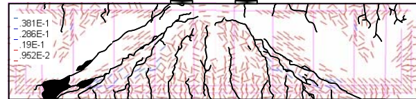
Fig.5.8. B10.3-1 crack patterns in different load steps (Test cracks are drawn with black lines).
