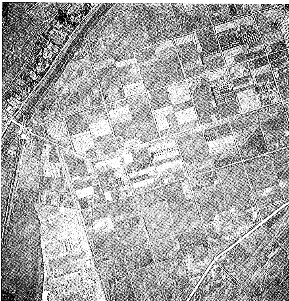
Photo. 8 Sand boils in the old riverbed of the Agano river during the Niigata Earthquake
