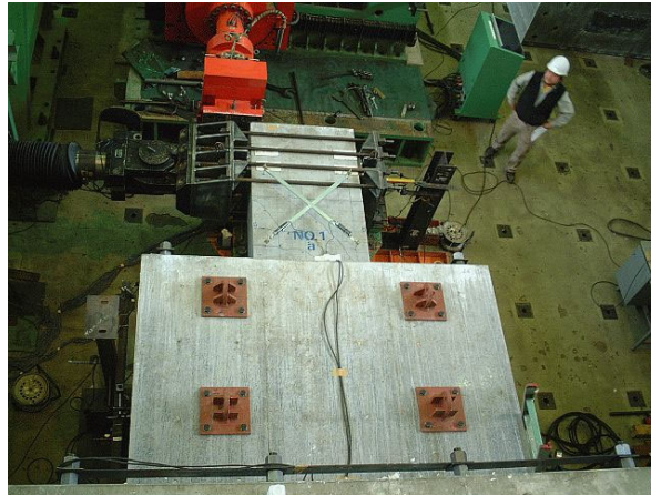
Photo-3.3.1 Example of Measurement of Shear Deformation
