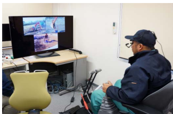
Fig.C-5 Cockpit type remote device
