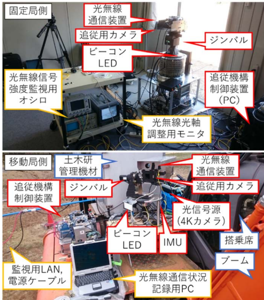
Fig.G-6 Mobile and fixed station settings
