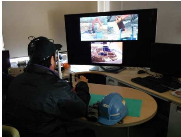
Figure.A-5 Remote control operation
