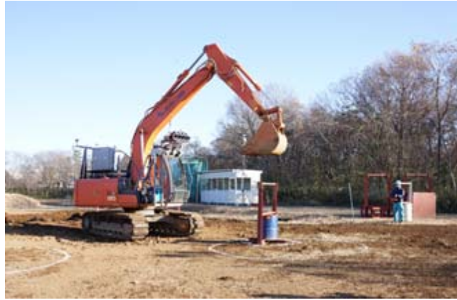
Fig.D-21 Remote operation on the ground
