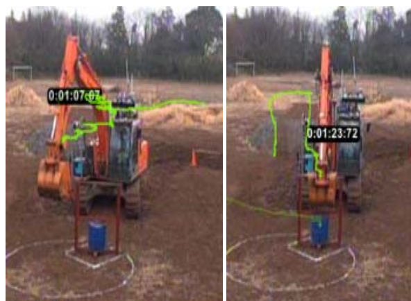
Fig.C-14 Operation analysis results (L: traveling R: grab)
