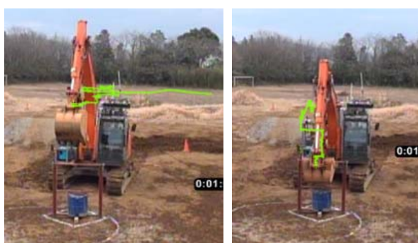
Fig.C-12 Operation analysis results (L: traveling R: grab)
