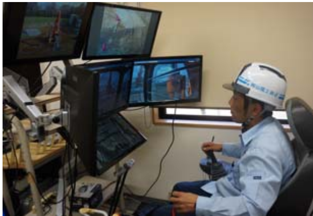
Fig.D-17 Operation with the cabin-type remote operation device
