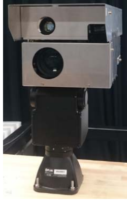
Fig. E-6 Free-space Optical Communication (FSOC) system
