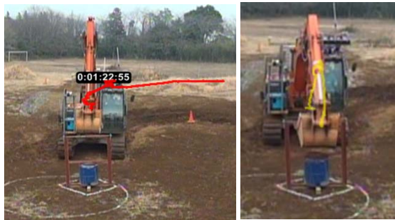
Fig.C-11 Operation analysis results (L: traveling R: grab)
