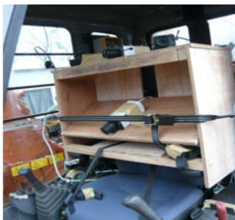
Fig.D-10 Camera arrangement
