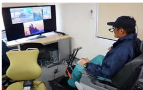
Fig.D-6 Operation with the cabin-type remote operation device
