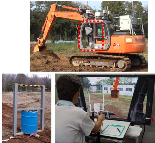
Fig. F-5 Video camera and remote control environment
