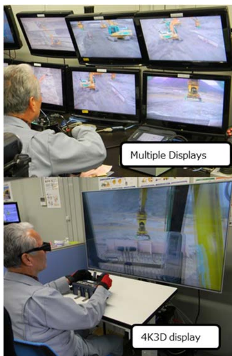
Fig. E-2 Remote Control Room
