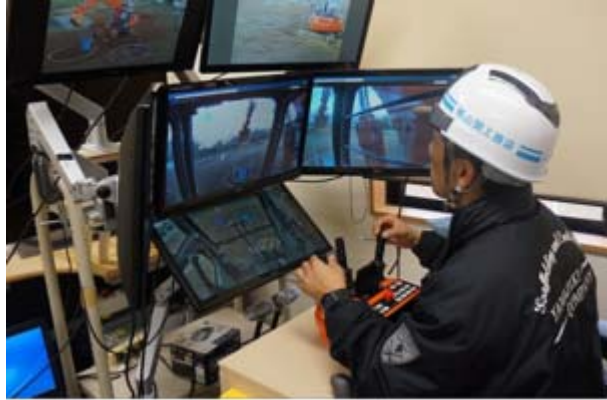
Fig.D-16 Operation using the conventional remote operation device
