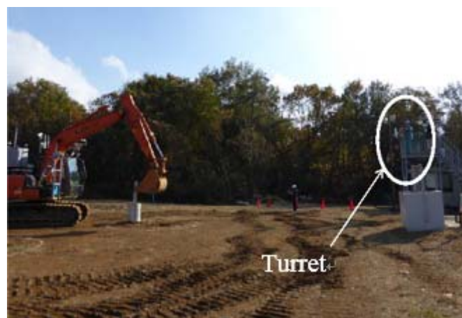
Fig.D-20 Visual remote operation from a high place
