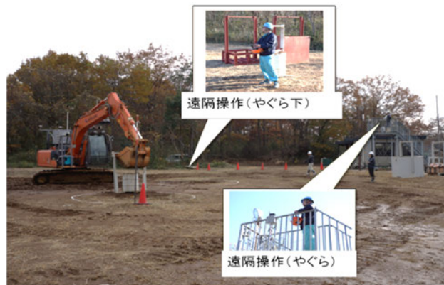
Fig.C-6 Remote control from the tower (visual)
