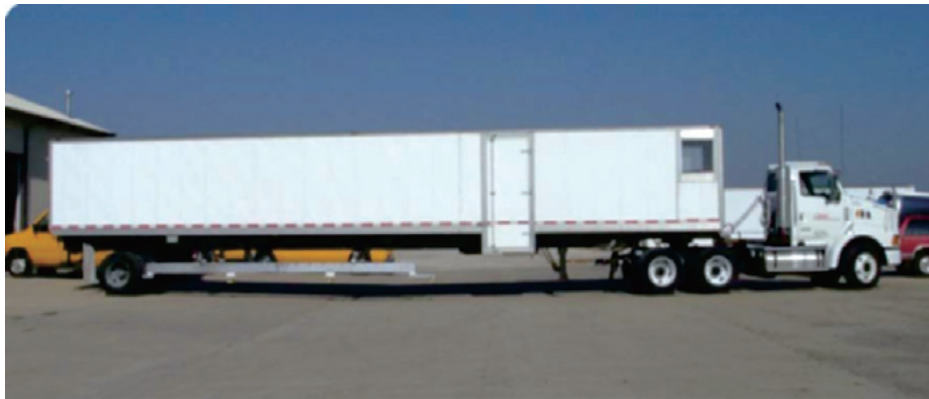
写真-1 RWD (Rolling Wheel Deflectometer (米国)) 13)
