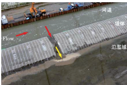
図-6 Step1 [初期破堤段階]
